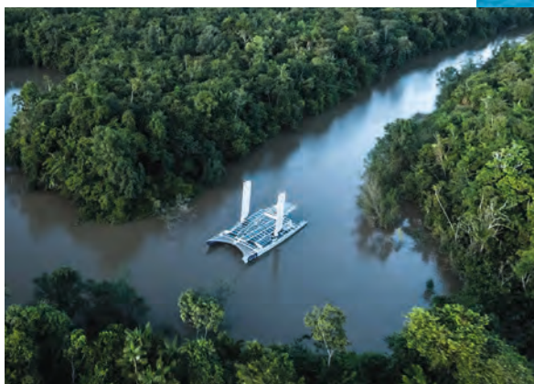
The Aqua concept by Sinot Yacht Architecture & Design and Lateral Architects suggests a possible set-up for 28 tonnes of liquid hydrogen powering PEM fuel cells (Render courtesy of Sinot Yacht Architecture & Design)
